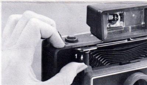
Pull camera front out as far as it will go.
